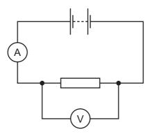
The reading on the ammeter is 2.0 A and the reading on the voltmeter is 4.0 V.
