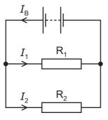
The current in the battery is  $I_{\rm B}$ . The current in R<sub>1</sub> is  $I_1$  and the current in R<sub>2</sub> is  $I_2$ .
